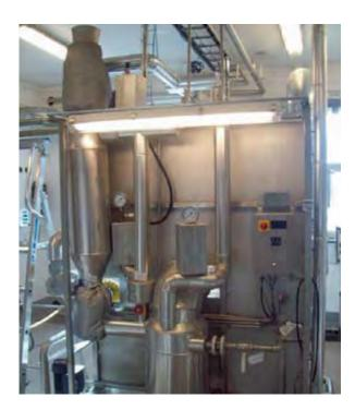
Figure 9: Pilot-scale steam explosion unit by CAMBI, Norway (photo by University of Natural Resources and Life Siences, Vienna, Division of Agricultural Engineering).
