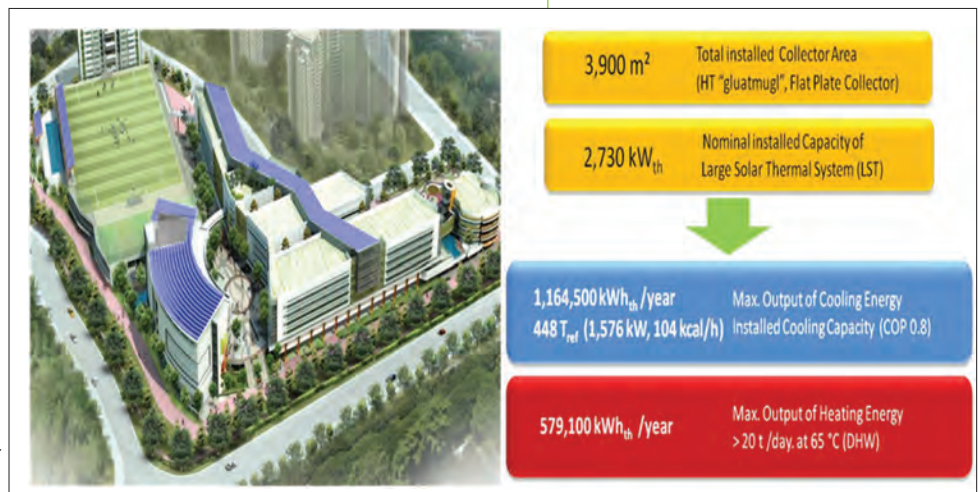
▲ Figure 1. Overview of UWCSEA solar thermal system
