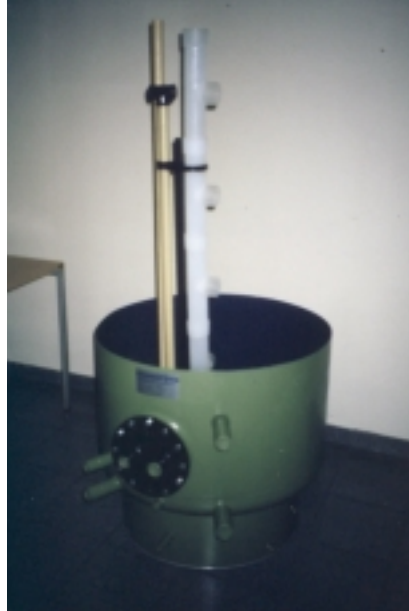
Fig. 13: Energy storage tank with the SOLVIS layer charging system (PINK)
