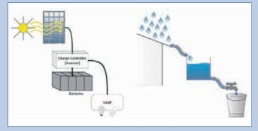
Fig. 5 - Simple analogy to explain energy storage system (from the above mentioned publication).
