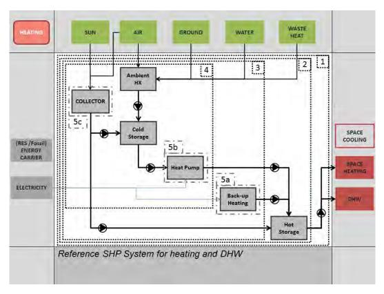
Figure 11: System boundaries for SHP Systems in heating mode
