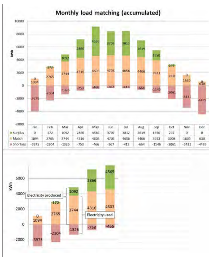
▲ Figure 3. The Sunscape Index tool is used during the early urban planning phase. It shows the outcome for the tested surfaces in terms of load matching: Green is the production of electricity beyond the need, Beige is the matched production, Pink is the lack of electricity. The user adds the profile of the building, the amount of square meters of useable area and surfaces at a certain angle and orientation. As seen in Figure 3, March to October are the primary months for solar energy production in Sweden.
