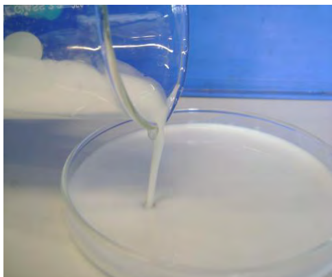
Figure 10: Paraffin/water-dispersion as phase change slurry for latent heat storage and transport
