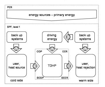
Figure 3: TDHP system boundaries for the definition of the performance figures
