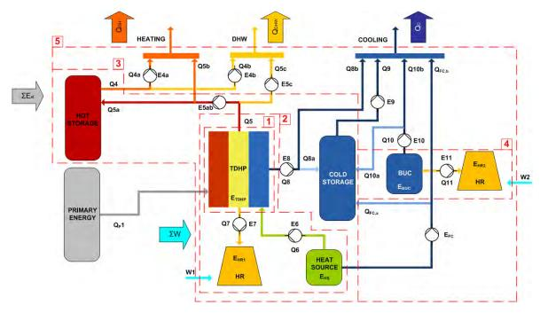
Figure 4: System configuration and boundaries for direct fired combined heating and cooling TDHP system
