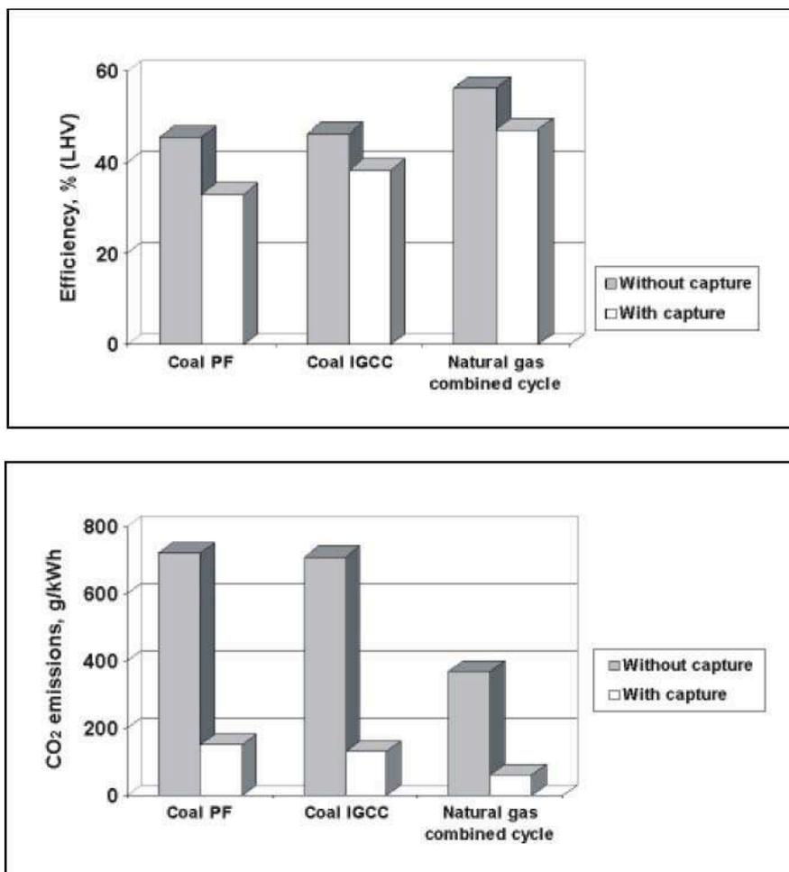
Figure 14: Power generation efficiencies and Figure 15: Power station CO<sub>2</sub> emissions
