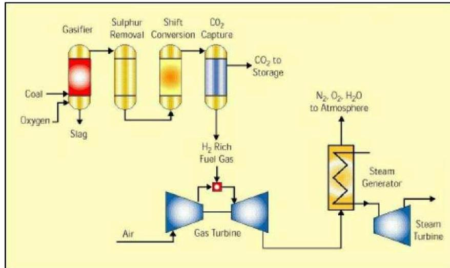
**Figure 6: Coal fired IGCC with pre-combustion capture of CO<sub>2</sub>**
