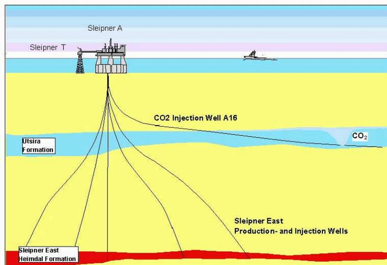
**Figure 5: Sleipner – CO<sub>2</sub> injection into the Utsira formation – courtesy of Statoil.**
