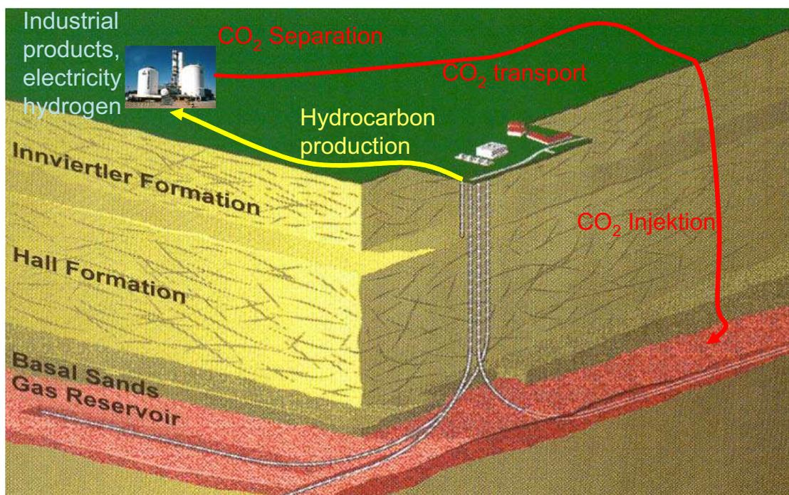
**Figure 4: Generating hydrogen and electricity without CO<sub>2</sub> emissions by using CO<sub>2</sub> geological storage: Hydrocarbons are produced from subsurface reservoirs, hydrogen and electricity is produced by conventional processes, CO<sub>2</sub> is separated from the flue gases and injected into reservoirs.**
