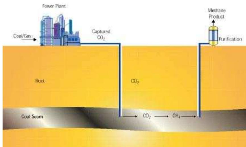
**Figure 13: CO<sub>2</sub> enhanced coal bed methane production**
