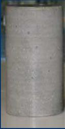
Neat cement: core after one month at 90deg.C-280 bars in Na<sub>2</sub>CO<sub>3</sub> solution (4%): perfectly preserved neat cement procedure not realistic in terms of severity criteria
