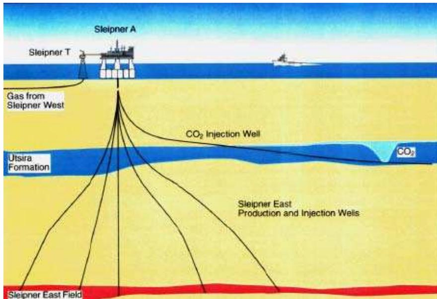
Figure 12: CO<sub>2</sub> injection into the Utsira deep saline reservoir (Courtesy of Statoil)
