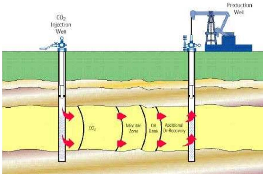
**Figure 10: CO<sub>2</sub> enhanced oil recovery**
