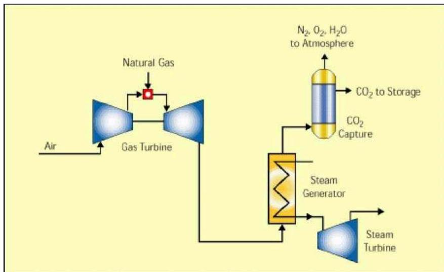
**Figure 5: Gas turbine combined cycle with post-combustion capture of CO<sub>2</sub>**
