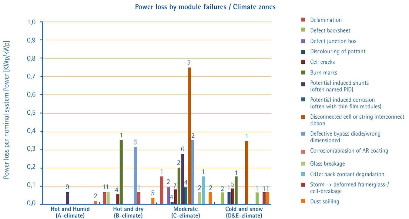
Fig. 3 - The power loss of various PV module failures is documented as a function of the climate zone (preliminary results). The columns' marking numbers count the occurrence of a specific failure type.
