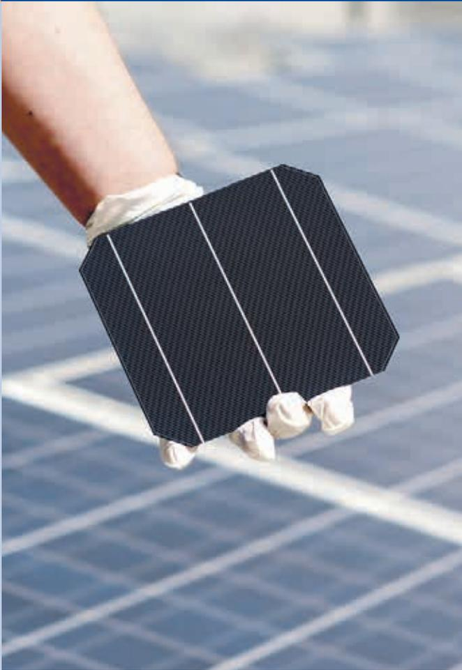
Fig. 2 - In January 2015, IMEC demonstrated a large area industrial crystalline silicon n-PERT solar cell with a record 22 percent efficiency.
