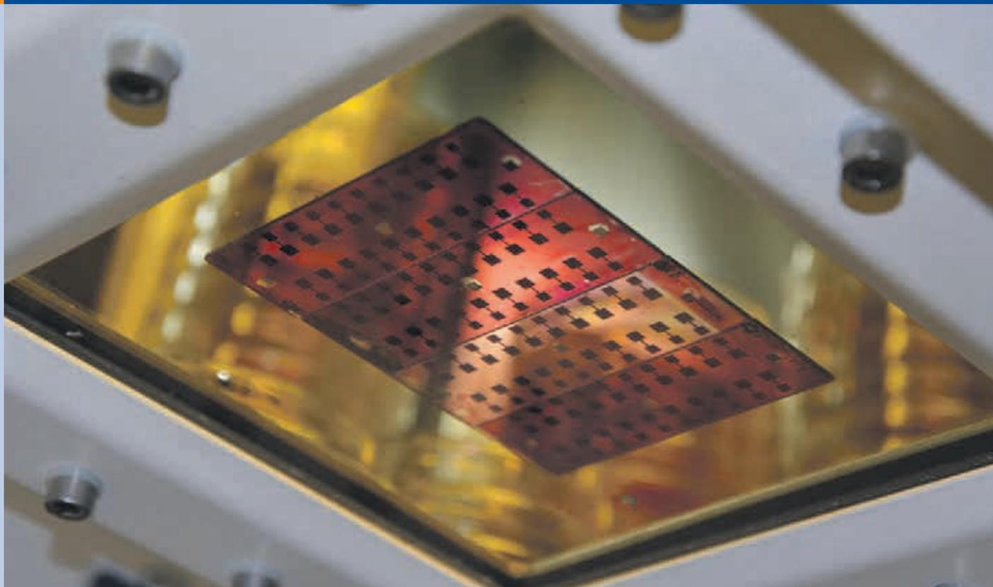
Fig. 1 - Laboratory test devices of inorganic-organic hybrid solar cells prepared at ICTM, TU Graz (Photo: © Astrid Knall, TU Graz).
