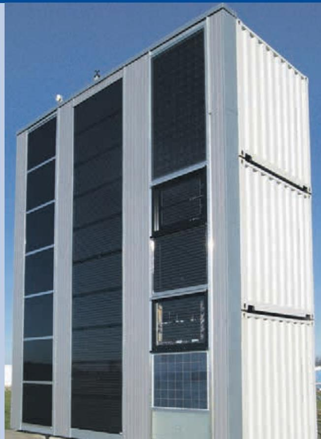
Fig. 1 – Test façade for various building integrated PV systems
