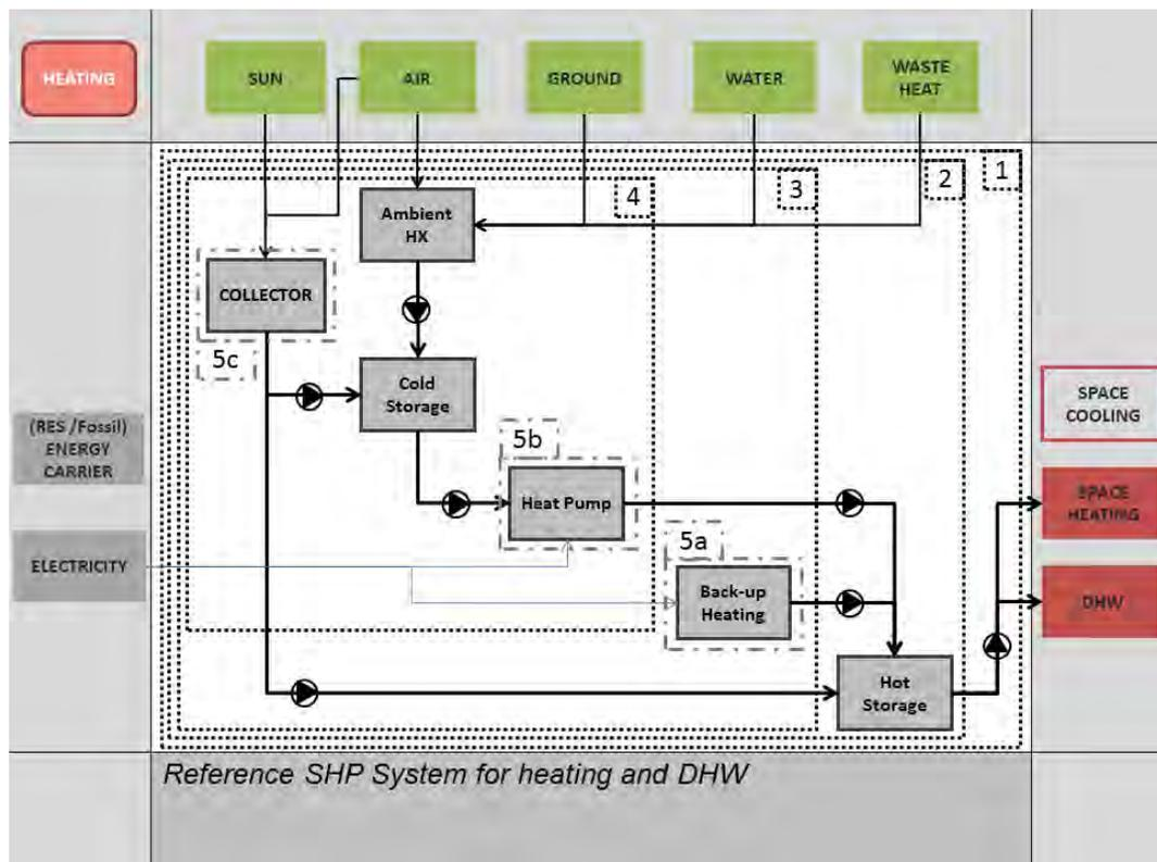
Figure 11: System boundaries for SHP Systems in heating mode
