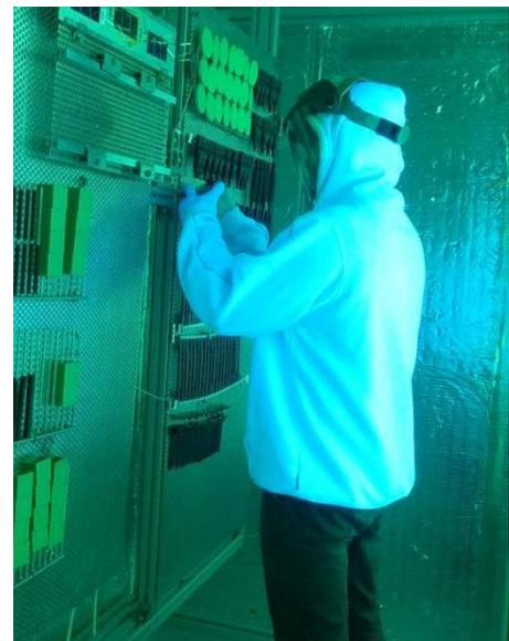
*Fig. 1 left: Comparison of the spectral intensity distribution of different light sources for UV aging. It shows not only a broad variation in total intensity, but also in regions of the UV range. Right: Researcher in protective gear sampling different polymer specimen in a UV chamber.*
