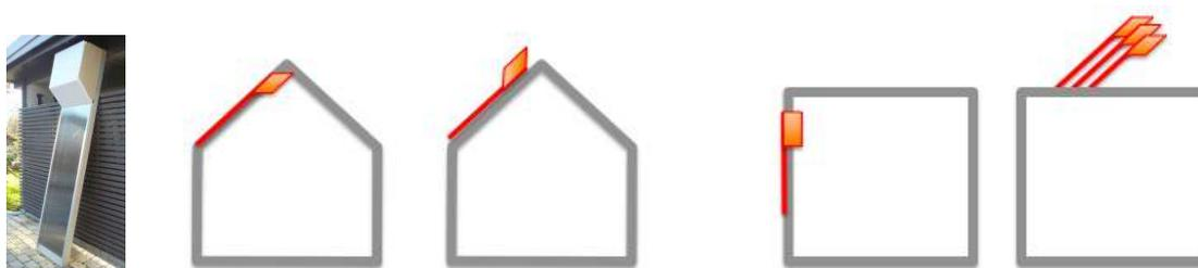
Fig. 3 – Different installation and integration options for the AventaSolar TSS concept.
